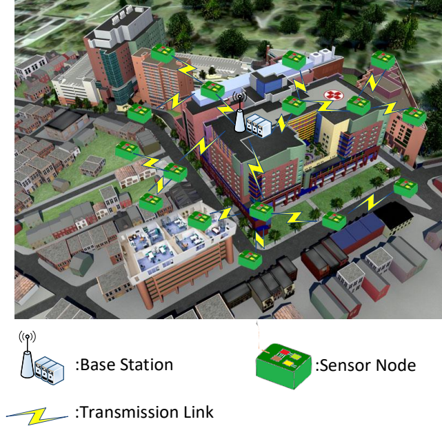
Fig. 1. The wireless sensor network application scene for hospital
